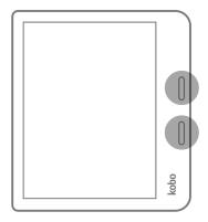
**To page forward and backwards:** Press the upper or lower page turn buttons. Depending on how you hold your eReader, the page turn button automatically adjusts so that the top button pages backward, and the bottom button pages forward.
